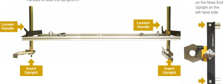
Then unscrew the 2 Nyloc Nuts M8 Flange on both Uprights and attach your guide bar as shown below. You may need to move the Nose End Upright towards the right if the guide bar you are using is smaller than the 64" GB Lo Pro Milling Bar shown.
