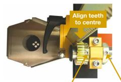
Check that both pinions are positioned correctly by looking at the position of the grub screws. If they are in the same position the bar is level.
