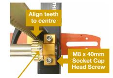
Check that both pinions are positioned correctly by looking at the position of the grub screws. If they are in the same position the bar is level.
