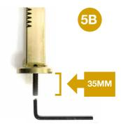
Add some thread locking compound to the M8 Grub Screws at the non Allen Key side and then screw them into the Rack Assemblies **leaving 35mm clear.**
