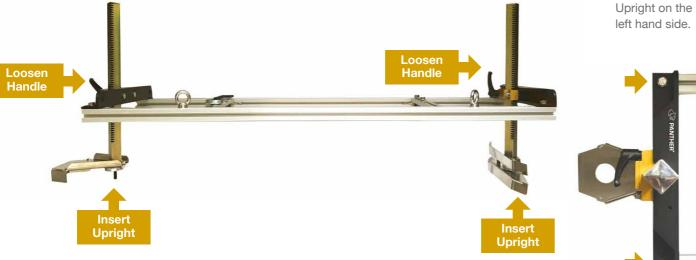
Then unscrew the 2 Nyloc Nuts M8 Flange on both Uprights and attach your guide bar as shown below. You may need to move the Nose End Upright towards the right if the guide bar you are using is smaller than the 42" GB Lo Pro Milling Bar shown.
