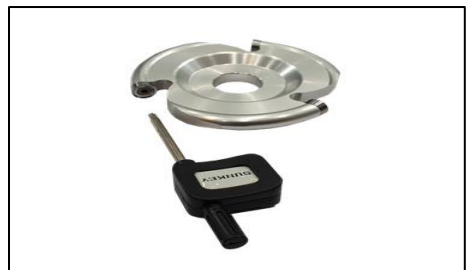
Image 2. Carbide teeth installed on the wheel
